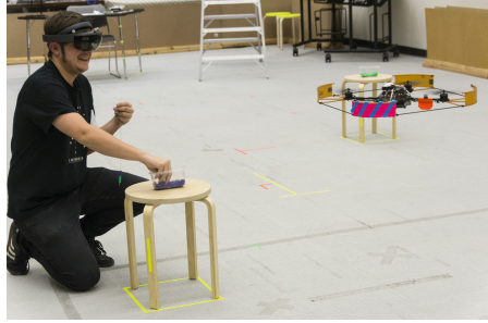
Fig. 5. We conducted a laboratory experiment to evaluate the effectiveness of our VAMR designs in improving human-robot interaction. Above, a participant wearing a HoloLens receives AR feedback informing him of the intentions of a nearby robot, helping to bridge a gulf of evaluation.
