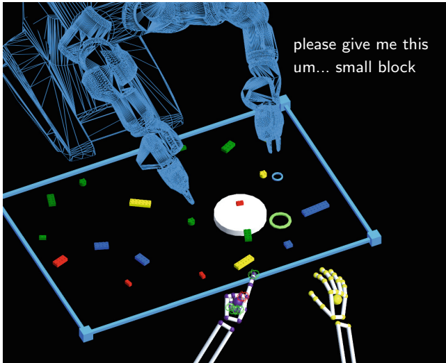
Fig. 4. Wizard interface with wizard's guess visualised as a white cylinder around an object. Multimodal input is represent as (a) text from speech recognition; (b) white rectangle being participant's head position and rotation, while a blue circle on the table surface is a projected vector from the centre of the head; (c) skeleton of a hand and a projected position from its finger on the table plane as a green circle. (Color figure online)
