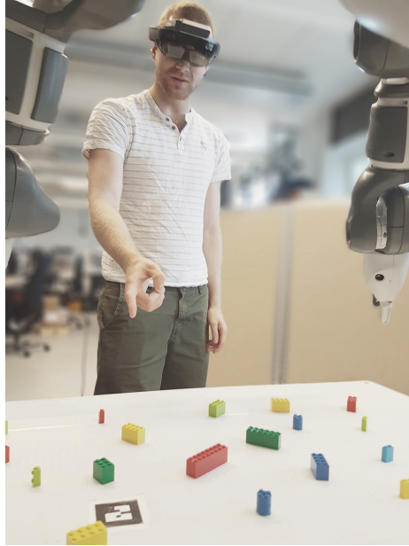
Fig. 1. Interaction scenario. The human agent is requesting a robot to give them Lego blocks. Any modality can be used in a natural way, no restriction to the interaction is applied. The only tracked modalities are head movements, hand gestures and speech. The participant wears a mixed reality headset to see which block to request and what is the robot’s estimation of their command.
