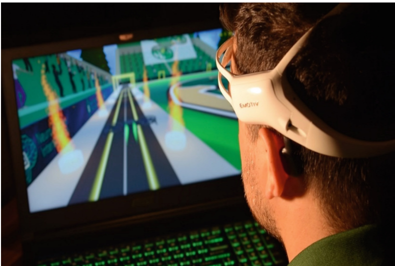
Fig. 1. Player controlling a virtual drone using a non-invasive brain-computer interface.
