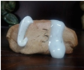
Fig. 1. Testing the temperature-measuring cone
