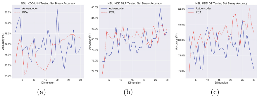
Fig. 9. NSL_KDD binary classification accuracy trends in the test set using the (a) kNN classifier; (b) MLP classifier; (c) DT classifier.
