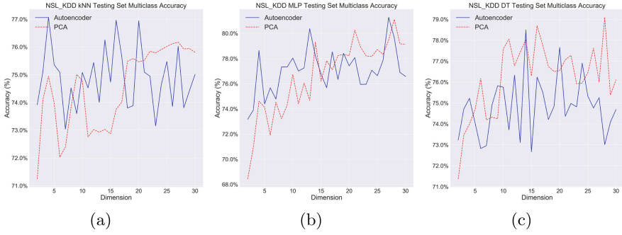
Fig. 10. NSL_KDD multiclass classification accuracy trends in the test set using the (a) kNN classifier; (b) MLP classifier; (c) DT classifier.
