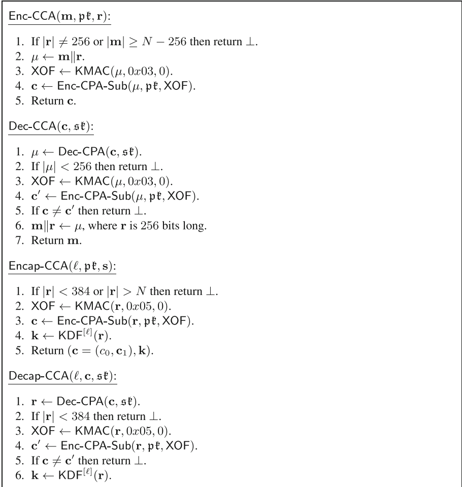
Fig. 2. CCA secure encryption, decryption, encapsulation and decapsulation algorithms for LIMA
