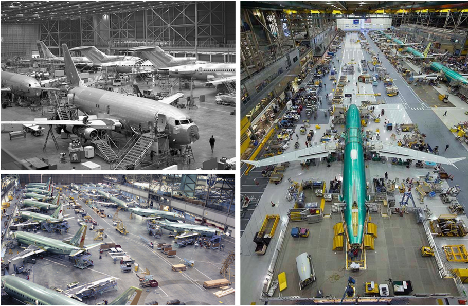
Fig. 5. The Boeing 737 final assembly, circa 1970 (top left), 1985 (bottom left) and at just prior to completion of the first 737 MAX, in 2015 (right)
