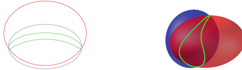
Fig. 2. Silhouette curves of two quadrics (in red and blue) and the cutcurve (in green)
