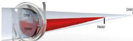
Fig. 2.2 Depiction of the focal points of a split bifocal
