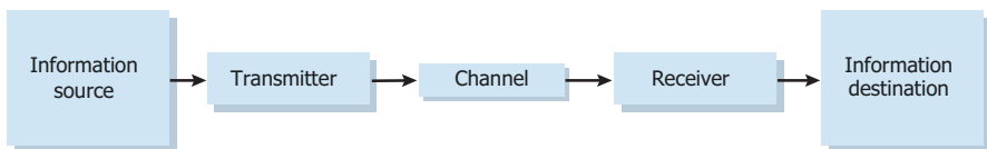
Fig. 12.2 Schematic diagram of the information system. (Modified from Shannon 1948)
