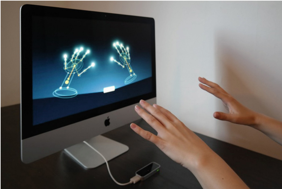
Fig. 2. A software application that shows hand and finger tracking by the Leap Motion (image taken from the official Web site).
