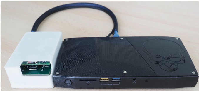
Fig. 11. A MOOCTab Box and a card reader for authentication.
