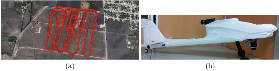
Fig. 2. Experimental field. To monitor the thermal radiance dynamics we instruct our UAS to follow an antipodal staggered flight several times over roughly the same area (a). For the flights we describe in this research, we use a 757-3 Ranger EX UAV (b). The FLIR Vue Pro-R camera mounted below the UAV’s fuselage.
