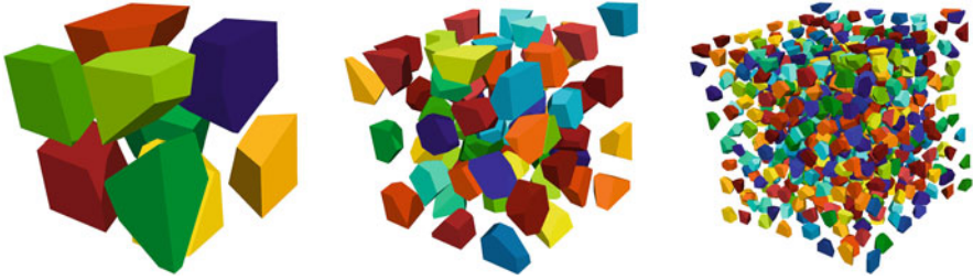
Fig. 6.8 Sequence of Voronoi meshes
