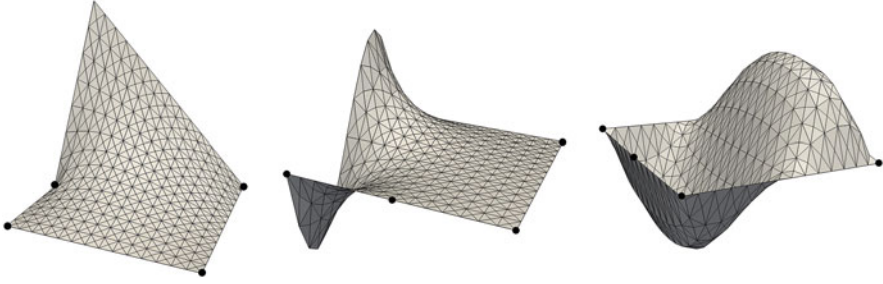
Fig. 2.10 Visualization of \psi_{\mathbf{z}} , \psi_{E,3} and \psi_{K,1,0} over rectangular element with additional node on straight line, nodes are marked with black dots
