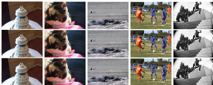
Fig. 2. Examples of cover images (top) and the corresponding steganographic images generated using LSB (middle) and SteganoGAN (bottom) with a relative payload of one bit per pixel. Both steganography techniques produce high quality images which, to the human eye, appear identical to the cover images.
