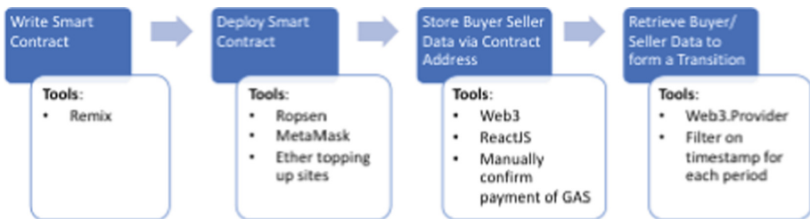
Fig. 3. Data storage and retrieval with Blockchain. Note: Tools listed here were used in this experiment, other tools could be chosen instead.
