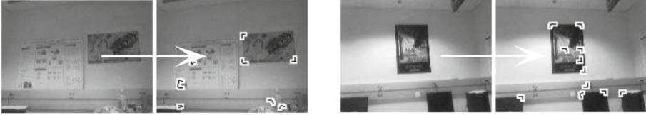
Fig. 1. The junctions detected using the JUDOCA operator.
