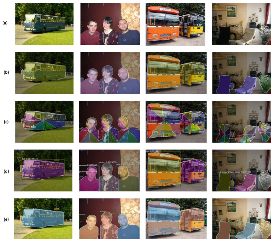
Fig. 4. Instance segmentation results. (a) Input image. (b) Semantic segmentation results. (c) Direction prediction results. (d) Instance segmentation results of our FSSI. (e) Instance segmentation results of MaskRCNN.
