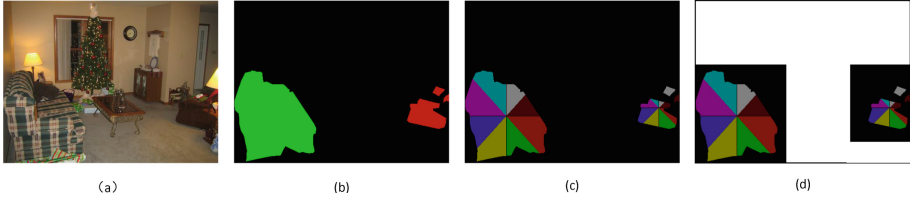
Fig. 2. Segmentation targets. (a) input image. (b) semantic segmentation target. (c) original direction segmentation target. (d) direction segmentation target after ignoring the background regions (in white color).
