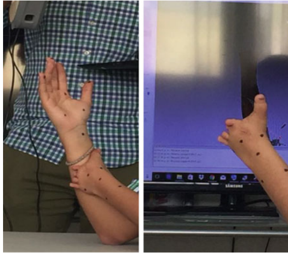
Fig. 38 Scan process of the patient’s left hand using ATOS Core and Artec 3D
