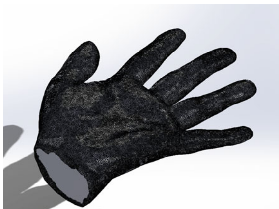
Fig. 36 Tridimensional model of the hand's structure after completing the previously mentioned steps. The archive was exported to the SolidWorks platform and can be appreciated as the conjunction of thousands of points
