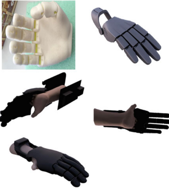
Fig. 40 Evolution of the prototype mechanism of the patient with tensioner and action mechanism
