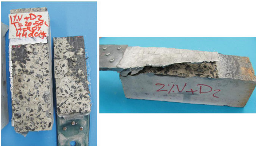
Fig. 10 Failure mode for tested CFRP/concrete samples after 44 days exposure using: a 1 wt% VGCF modified DGOA (left), and b 2 wt% VGCF-modified DGOA (right)
