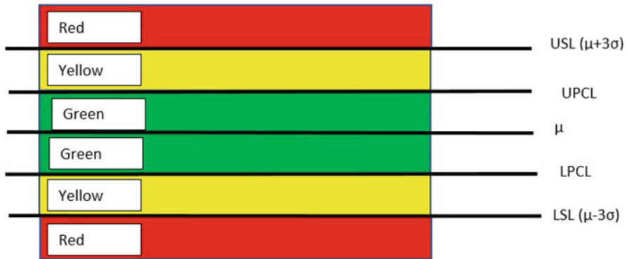
Fig. 1 The basic set-up of pre-control chart
