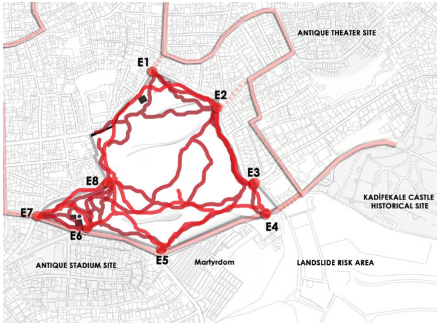
Fig. 7 Superposition of the thickest routes of the shortest paths of live plasmodium
