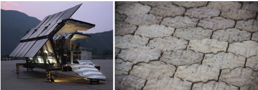
Fig. 1 Trashpresso [4], a Trashpresso mobile, plastic recycling plant, b upcycled architectural tiles from waste plastic using Trashpresso
