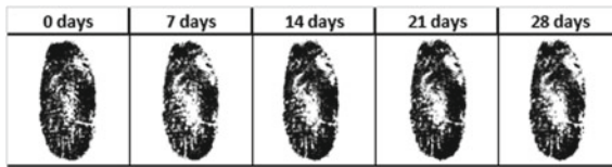
Fig. 3.14 Visible ridge detail for blood-stained fingermarks analyzed using HSI after zero, seven, fourteen, twenty one and twenty eight days. Reprinted from ref. [79] with permission from MDPI
