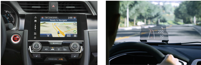
Fig. 1. Examples of navigational displays in modern vehicles (left: head-down display; right: head-up display) [5, 6].
