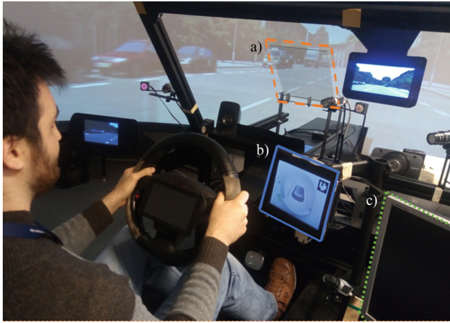
Fig. 1. DSM: (a) Head-up display (orange dashed outline); (b) Assistive cluster interface (blue solid outline); (c) Touchscreen display (green dotted outline).
