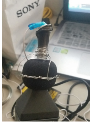
Fig. 4. Image of an earphone attached to the ear canal model
