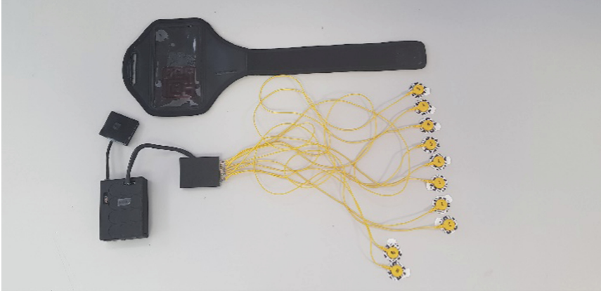
Fig. 5. Device for sEMG signals capture.
