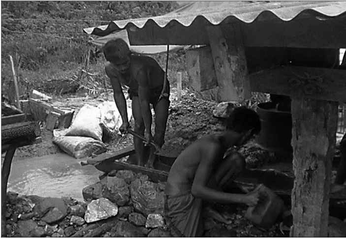
Fig. 2. Compressor mining process showing miners sluicing the mud to separate gold from dirt
