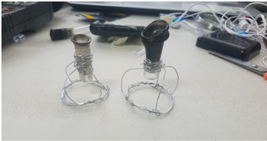
Fig. 3. Ear canal models used to benchmark the sound derived from the earphones
