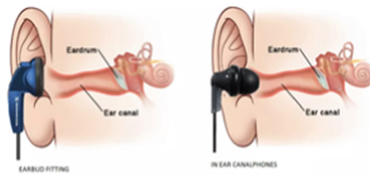
Fig. 1. Illustration of the earbud type earphones (left) and the in-ear/canal type earphones (right) [4].
