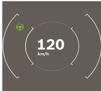
Fig. 3. Example of the centre of the Head-Up Display (HUD) with AD mode engaged.
