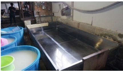
Fig. 7. Sukibune. Bath to keep dissolved stock to comb the paper.
