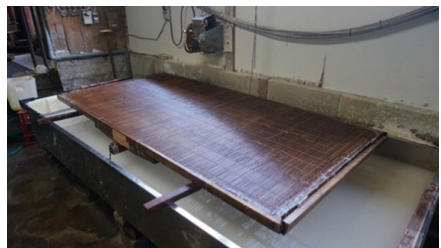
Fig. 8. Sukisu. Equipment which scooped the paper stock solution to form a paper layer thereon from “Sukibune”. The lottery shaved round thin bamboo is a Takesu braided tail hair of silk or horse.
