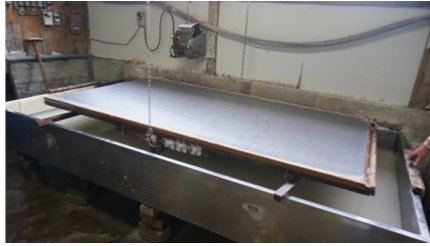
Fig. 9. Sugeta. A tool that supports the “Skisu” and raises paper. The combination of “Sukisu” and “Skigeta” is called the “Sugeta”.
