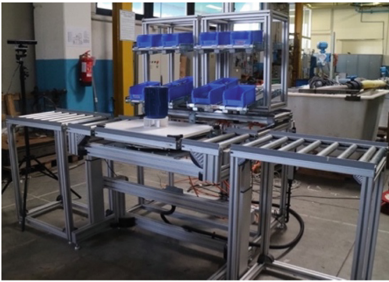
Fig. 1. Assembly workstation used in this study. The workstation consists of three roller conveyors (one in the central position and two lateral) and a metallic frame. Two front modules contain the boxes with the parts and components for the assembly task.
