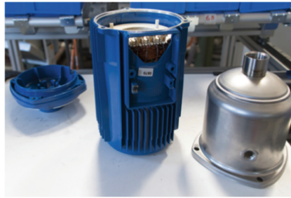
Fig. 2. Parts of the horizontal multistage centrifugal electric pump. From the left: seal housing disk, pump crankcase, lantern.
