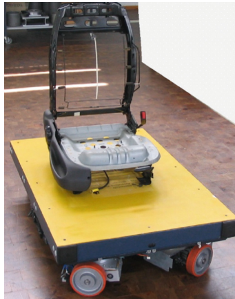
Fig. 5. AGV applied to transportation of the seat frames.
