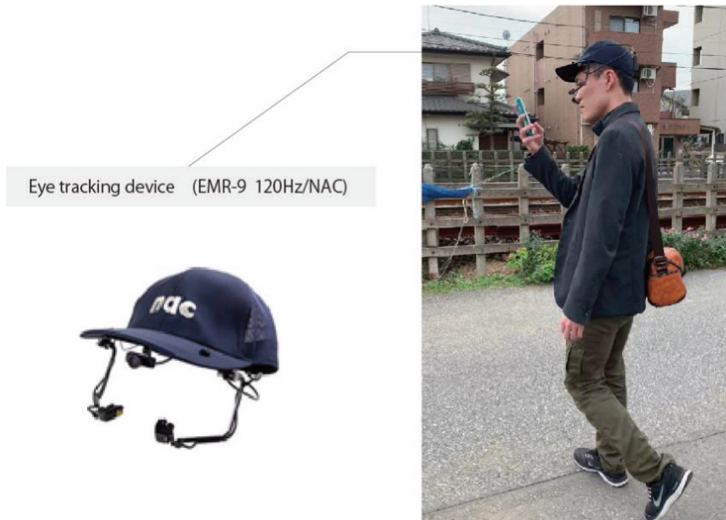
Fig. 3. Experimental equipment. The subjects wore the 120 Hz eye tracking device (EMR-9/NAC) so that the subject's gaze position while walking on the route could be detected.
