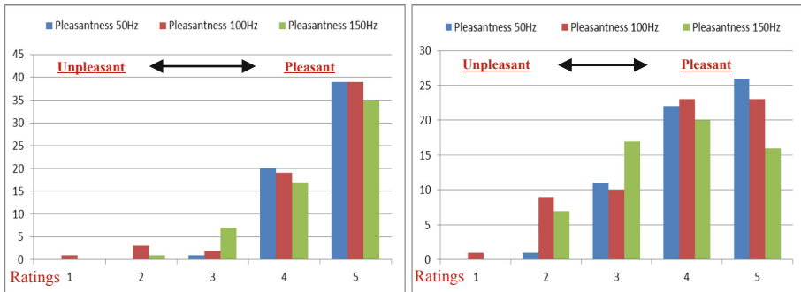
Fig. 8. Subjective ratings of pleasantness for the applied signals averaged over 20 participants over the three frequencies and delay parameters for HM-Glove (left) and Haptic Glove (right).
