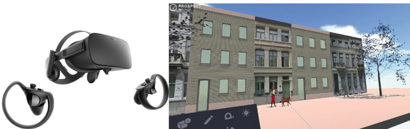
Fig. 5. VR test setting: Oculus rift VR-goggles and controls (left) and VR test environment (right).
