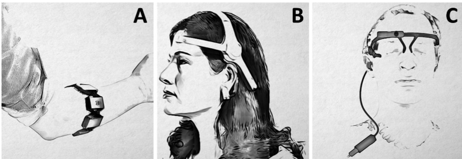
Fig. 2. The products utilized in the study: Gesture controller (A), a Brain-Computer Interface device (B), and eyewear integrating gaze tracking (C).
