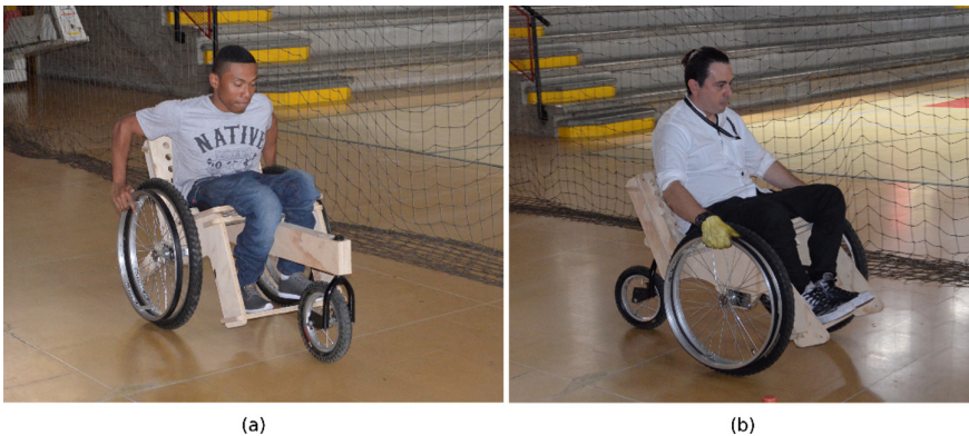
Fig. 1. Plywood functional models used to test the position of the caster wheel in (a) front position and (b) rear position.
