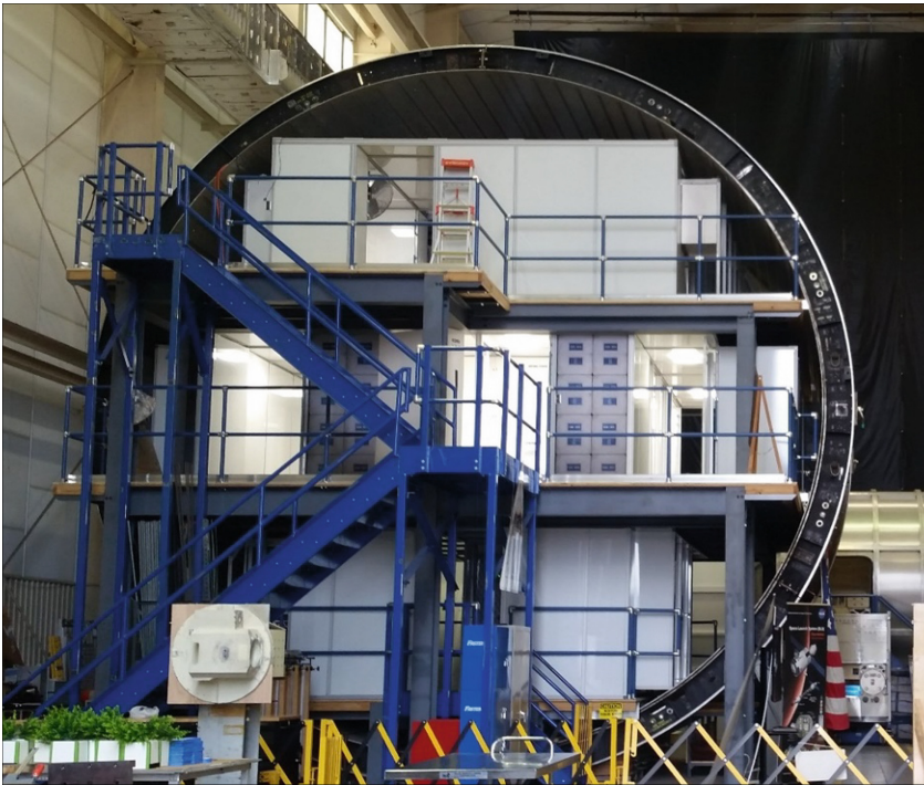
Fig. 2. The physical SLS derived Deep Space Habitat (DSH) mockup. This mockup includes a galley and exercise area on the upper deck, crew quarters and laboratory equipment on the mid-deck, and a work area on the lower deck.
