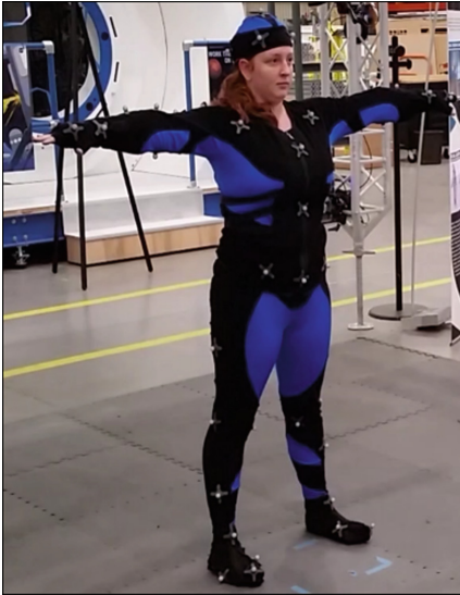
Fig. 7. A participant using the MoCap system wearing the Vicon suit and trackers.
