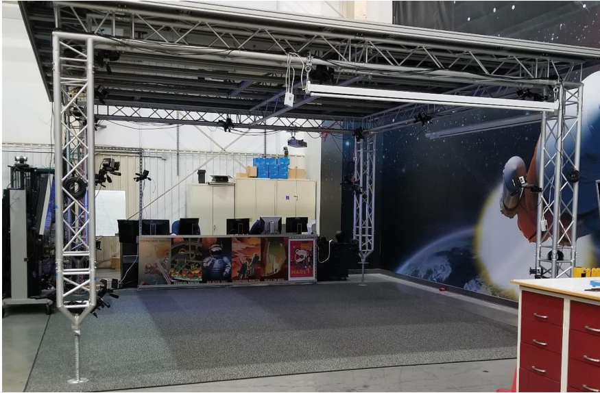
Fig. 1. Virtual Environments Lab (VEL) at NASA Marshall Space Flight Center. The VEL contains a 16 infrared Vicon motion capture camera system and VR capabilities with Oculus Rift and HTC Vive.
