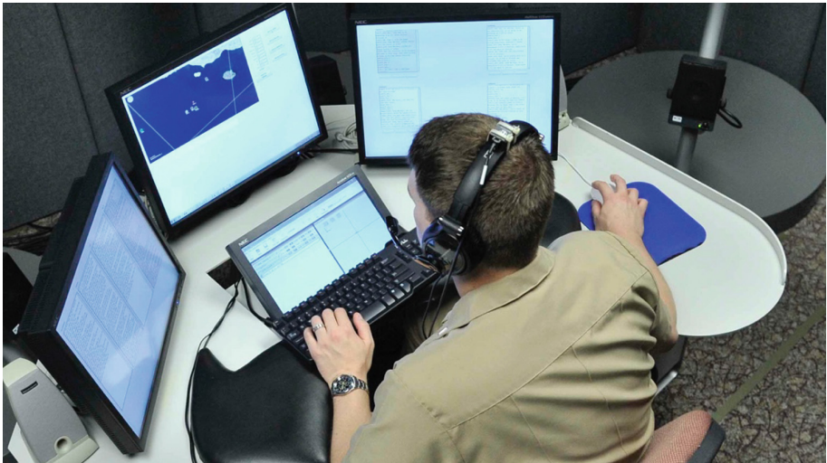
Fig. 3. The TFS being used to explore mediated management of user attention in a highly multi-tasked, simulated command-and-control information environment.
