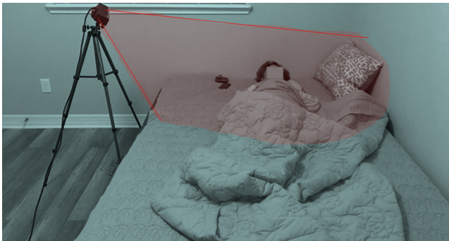
Fig. 1. In-home experimental setup: MS Kinect II depth sensor.
