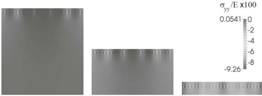
Fig. 5.18 Dimensionless vertical contact stress \sigma_{yy} in the continuum depending on the domain size, t , for a far-field imposed displacement w/A_0 = 3 (WM rough profile with D = 1.25 , \gamma = 5 , n = 2 , see Fig. 5.3 for the visualization of half profile). Adapted from Paggi and Reinoso (2018)
