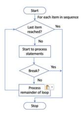
Typically, a guard statement (if statement) is placed on the break so that the break statement is conditionally applied when appropriate.
