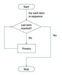
This flow chart shows that some sequence of values (for example all integer values between 0 and 9) will be used to iterate over a block of code to process. When the last item in the sequence has been reached, the loop will terminate.
