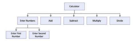
We might also identify the need to determine which numerical operation should be performed based on user input. This function might sit above the numerical functions or along side them. This is in fact an example of a design decision that the designer/developer must make based on their understanding of the problem and how the software will be developed/tested/used etc.
