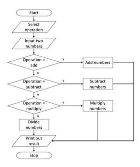
The above flowchart shows the basic operation of the calculator; the user selects which operation to perform, enters the two numbers and then depending upon the operation the selected operation is performed. The result is then printed out.
