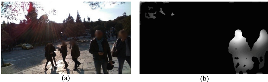
Fig. 7. Example detection of high risk obstacles (nearest crowd and tree branches). (a) Original image RGB image. (b) The corresponding image O_{obstacle}^1 obtained by using membership function d_I .
