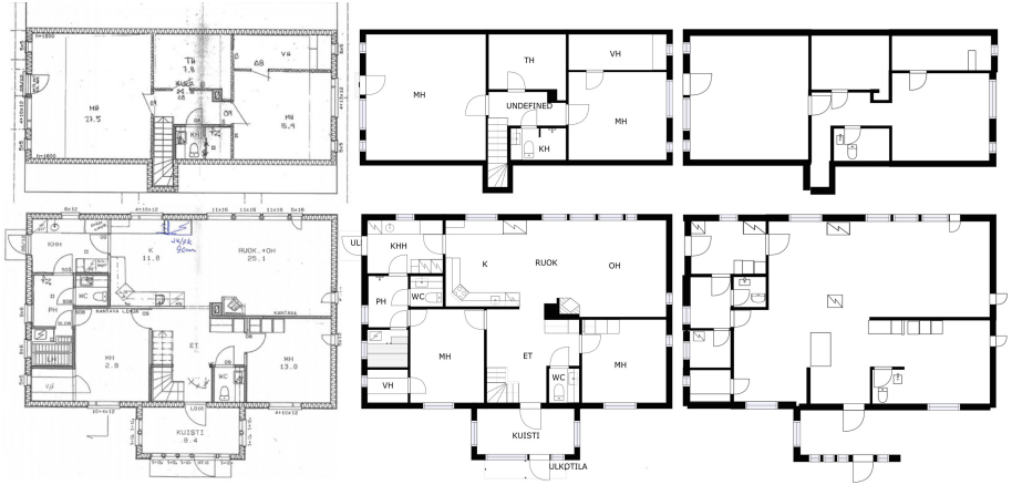
Fig. 1. An example result using our dataset and pipeline. The images from left to right are original floorplan image, the SVG label, and the automatic prediction.
