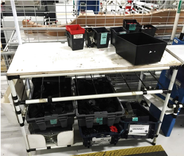
Fig. 3. Workstation before distribution changes. Workstations show, initially, disorder, changes on workloads, lack of identification in materials containers and workstation itself, visual control.
