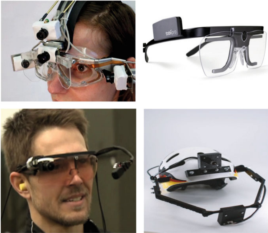
Fig. 13.7 Top left, The EyeSeeCam (Kohlbecher et al., 2010) with two scene cameras, one of which moves with the eyes to keep it aligned with the current direction of gaze. Top right, a Tobii mobile eye tracker with two cameras for each eye and a scene camera. Bottom row, Research-based eye trackers used for a skeet shooting and whitewater kayaking experiments, designed and built by researchers at IT University of Copenhagen for these purposes
