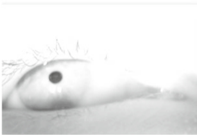
(C) Bright daylight floods scene camera and obscures corneal reflection of IRLED
