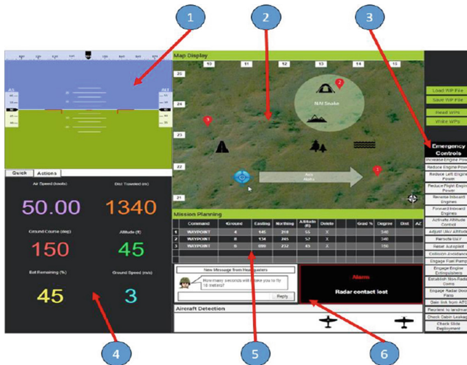
Fig. 1. Prototype interface - (1) primary flight display (PFD), (2) mission map, (3) emergency controls, (4) flight parameter display, (5) waypoint display table, (6) mission task bar.
