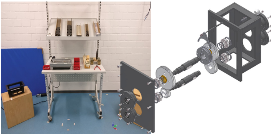
Fig. 1. Workplace setup for motion recordings of an assembly task (left) and the assembly object (right)
