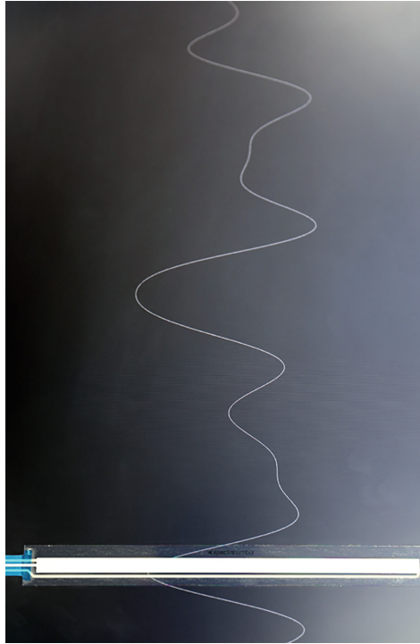
Fig. 3. For pursuit tracking, the gesture waveform moved down the screen toward the touch strip, and the subject was asked to move her or his finger along the touch strip in synchrony with the waveform as it moved downward.
