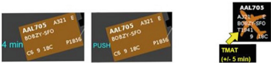
Fig. 3. Flight strips for aircraft in both metering conditions: (left) at gate showing gate hold advisory countdown (“4 min”) to the TOBT (Target Off-Block Time); (middle) at which time “PUSH” is indicated; (right) after pushback with TMAT (Target Movement Area entry Time) showing “1941” for arrival at the spot.
