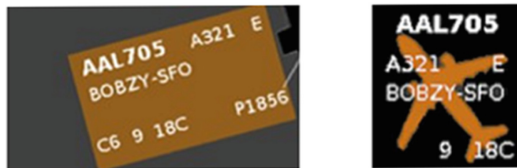
Fig. 2. Digital flight strips on the RTC display in the baseline, or no metering condition, (left) at the gate prior to pushback and (right) following pushback, while taxiing in the ramp area.
