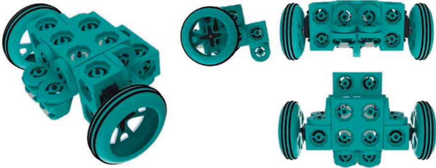
Fig. 5.28 Mobile robot follows-lines, two-wheel drive
