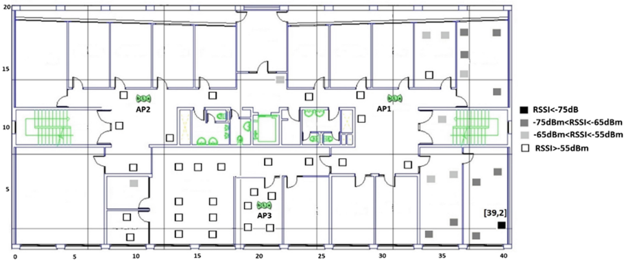
Fig. 4. RSSI measurements obtained before the AP Relocation i.e. AP3 at [20, 4] .
