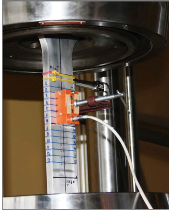
Fig. 38.1 Measurement of acoustic anisotropy: 1—corset sample in the test machine, 2—IN5101A device with piezotransducers
