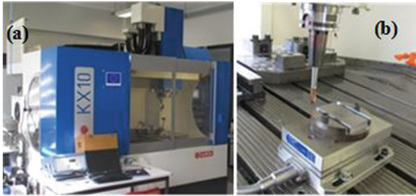
Fig. 4. Experimental setup (a) Huron center KX10 (b) Tool/Workpiece/Kistler dynamometer
