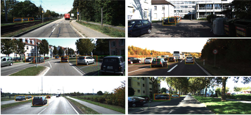
Fig. 6. Sample car detection improvement with AR estimation on KITTI-train10. In green, red and yellow we show respectively the ground truth, Estimated-AR-Mean and Fixed-Class-Mean true positives for the data base moderate settings. (Color figure online)
