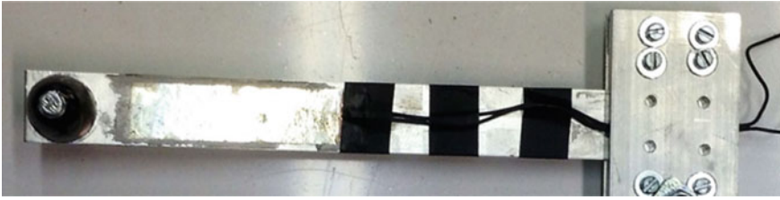
Fig. 4 Piezoelectric cantilever for energy harvesting (Cahill et al. 2018)
