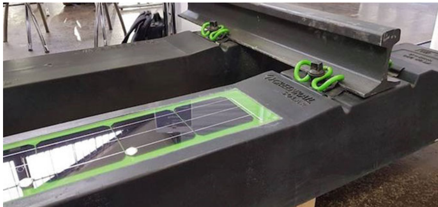
Fig. 8 Solar sleeper (Greenrail Project No. 738373—H2020-SMEINST-2-2016-2017)
