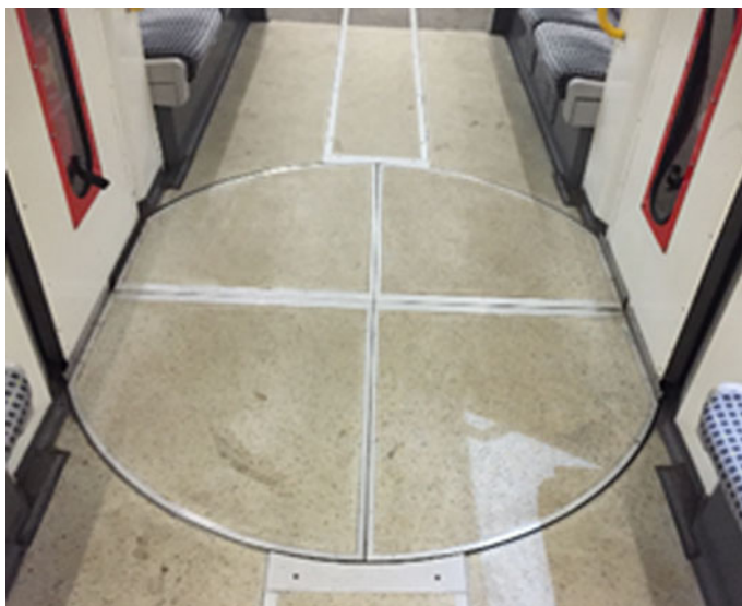
Fig. 7 Centre section of metro facilitating a pivoting bogie
