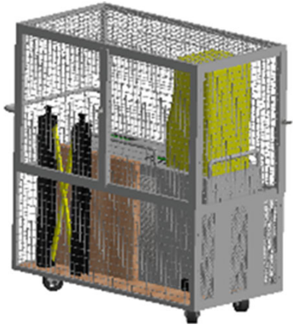
Fig. 53 Roll container with equipment stored within it
