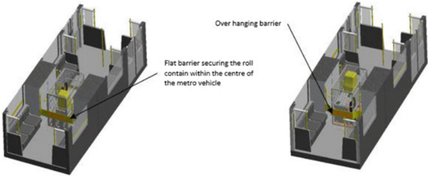
Fig. 54 The check-in and bag drop facility packed away for Design 2.2
