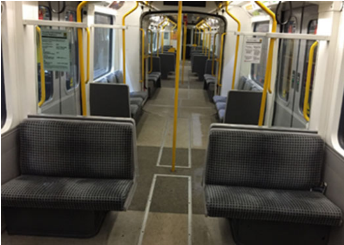
Fig. 11 Differing width of aisles between the centre of metro and standard seating
