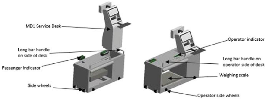
Fig. 38 Explosive view of Design 2.1 check-in desk
