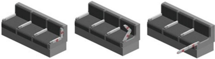
Fig. 30 Set up of double jointed fold out arm to act as barrier
