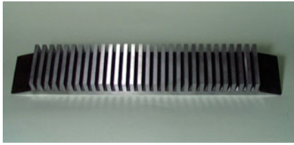
2-D fence 60mm × 300mm, height 20mm
