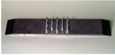
Arrayed cones having 15mm base diameter, 30mm high
