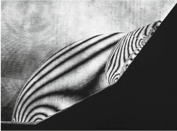
Fig. 2.73 Apparent StMR over a 30^\circ/55^\circ double wedge: #87120719, for Ms = 1.927 in air at 500 hPa 293.0 K, the first wedge length of 50 mm
