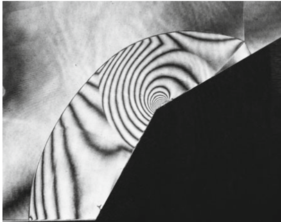
Fig. 2.84 Reflection of a MR over a 60^\circ/30^\circ convex double wedge: #86012709 630 \mu s, Ms = 1.498 in air at 670 hPa, 288 K
