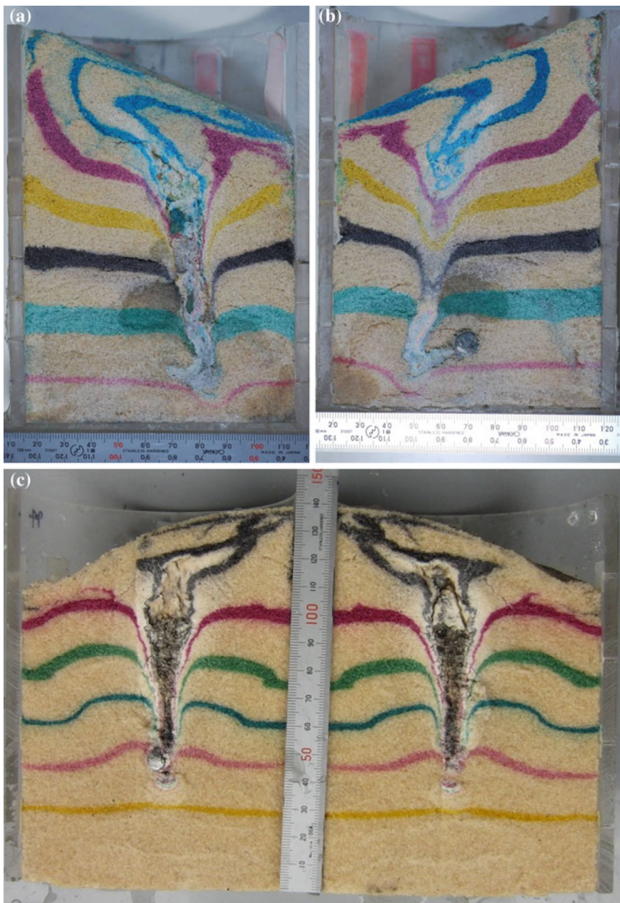
Fig. 11.28 Penetration of sphere into sand layers: a, b impact against oblique surface at 1.93 km/s: c #11030201, 1.02 km/s; d #13032901, 1.01 km/s; e enlargement of (d) (Yamamoto et al. 2015)
