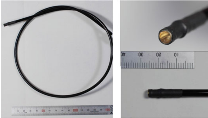
Fig. 10.41 Prototype of a shock wave ablation catheter (Yamamoto et al. 2015)
