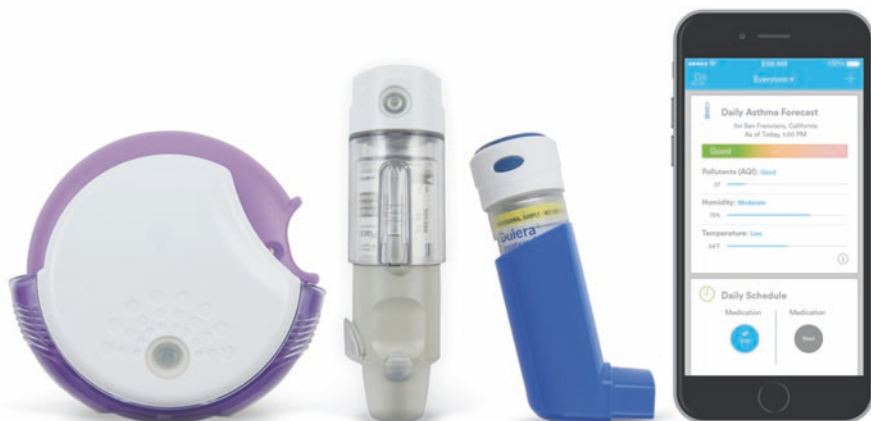
Fig. 2 Data on the timing and frequency of medication use are transmitted wirelessly via a paired smartphone or hub to Propeller’s HIPAA-compliant servers. The platform, comprising smartphone apps, web dashboards, and other communication channels, presents findings and education to participants and clinicians
