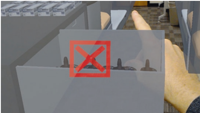
Fig. 6 Notification that indicates the false selection of an object/equipment and thus unsuccessful completion of a task
