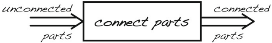
Fig. 7.7 Black-box model to describe the overall function of a glue gun [GeEi-2017]
