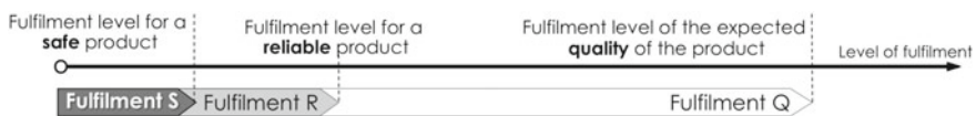
Fig. 3.6 Levels of fulfilment with the fulfilment attributes safety (S), reliability (R) and quality (Q)
