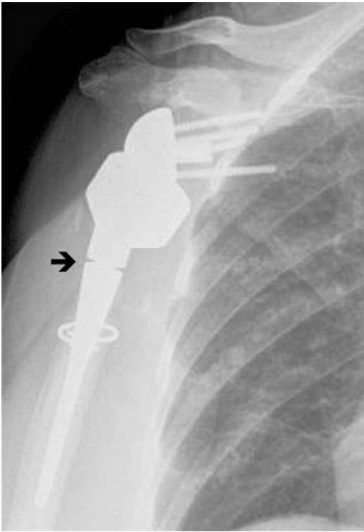
Fig. 20.8 Grashey view of RTSA with demonstrating dissociation of the distal humeral stem from the proximal metaphyseal modular component. Black arrow points to gapping between metaphyseal modular component and humeral stem, which should not be present
